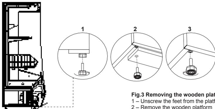
**Fig.3 Removing the wooden platform**
